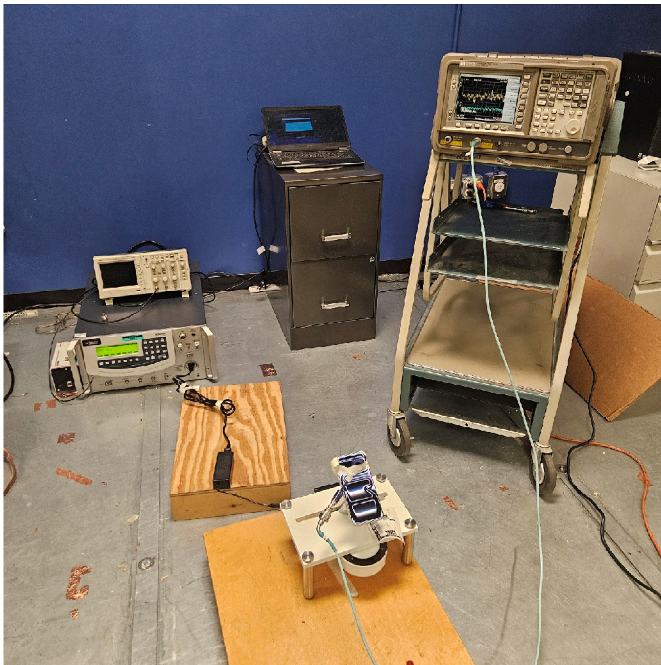
Photo 2.5.8-1 – EFT Test Setup, AC Power Ports
