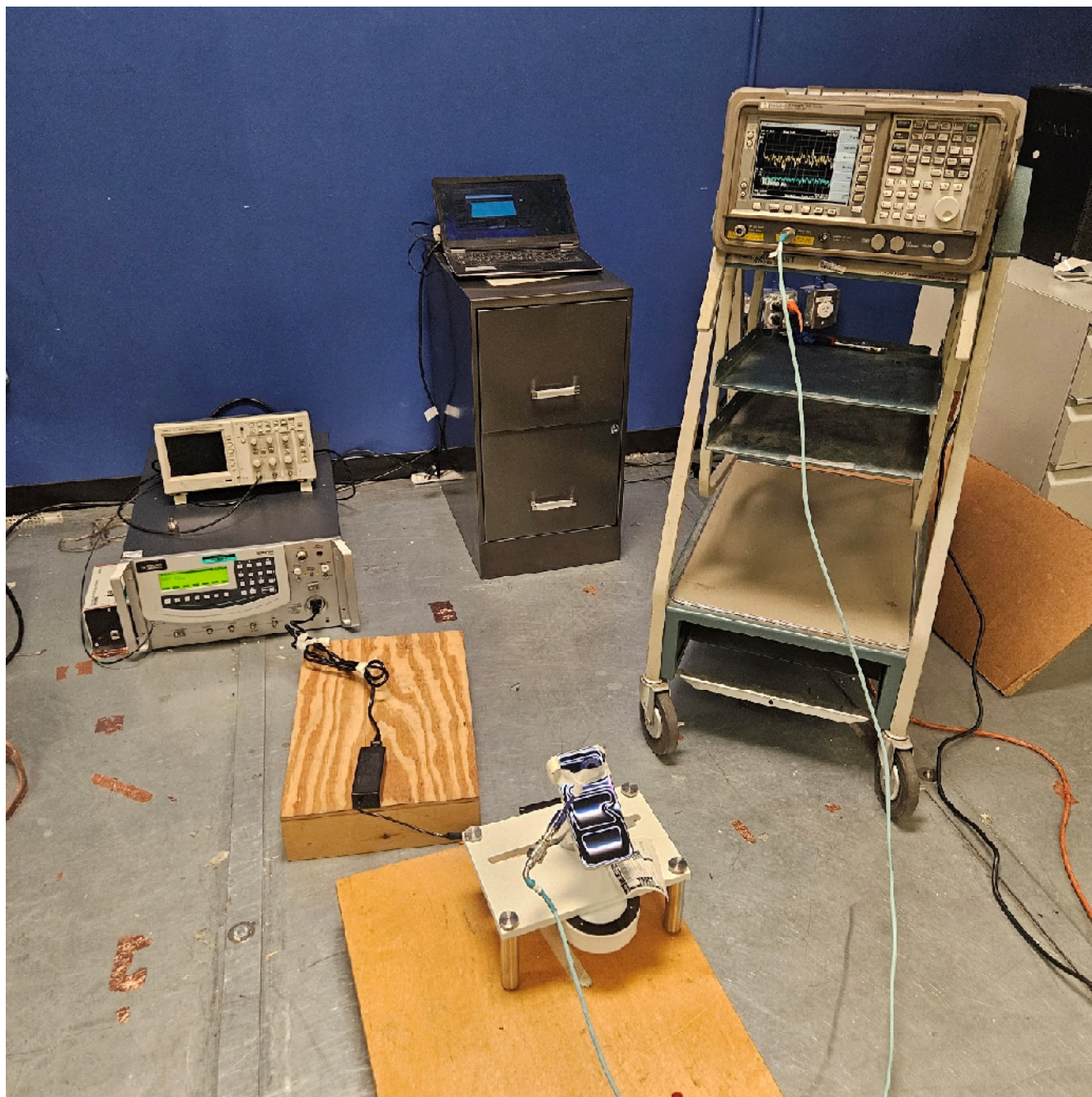
Photo 2.6.8-1 – Surge Test Setup, AC Power Port
