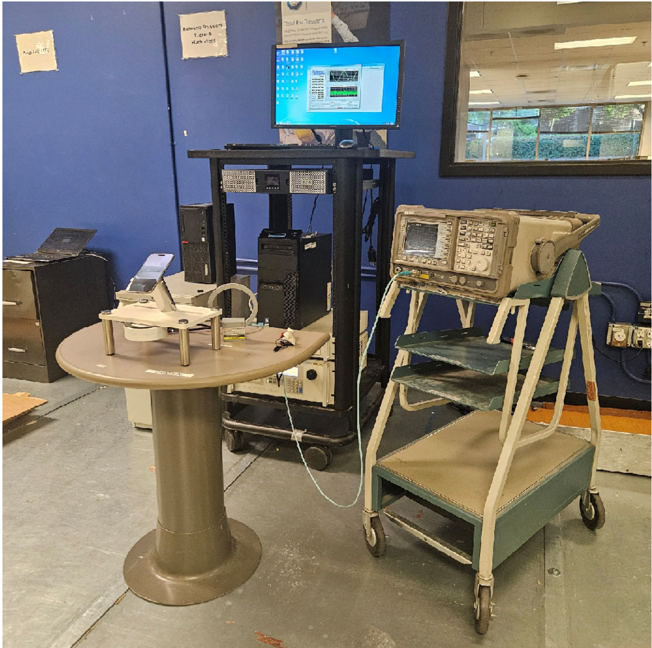
Photo 2.10.8-1 – Harmonic Current Test Set-up
